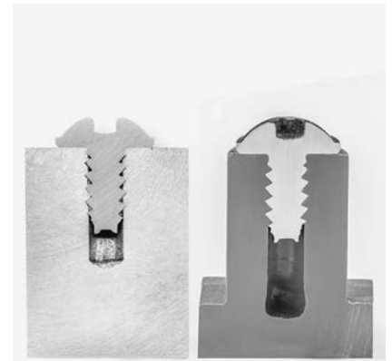
High flank coverage can be achieved for screw connections in light metal casting alloys and plastics
